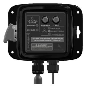
The alarm status will continue as long as fume levels remains at an elevated level. The alarm horn may be silenced by pressing the "Silence" button. The problem should never be considered corrected as long as the Red LED is illuminated.
